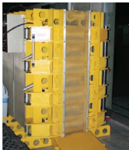
This wheel cage was designed with the assistance of military experts with experience of mine resistant vehicles. If a tyre explodes during inflation, the blast is dissipated and debris contained (photo: myTECHNIC)
